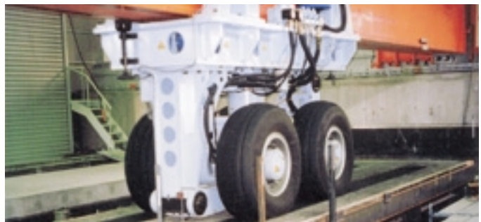
Photo 8 Durability test on pavement of floating airport runway model
