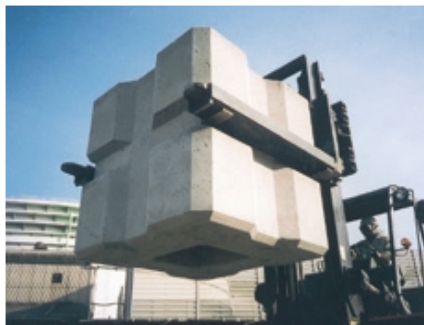
Photo 1 Coal-ash cement block (a 1.6 m cube weighing 6 tons) being moved with a forklift truck
