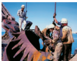
Photo 2: Cutter Head Source: References 3)
