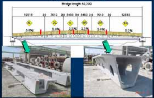
Pre-cast blocks assemble
