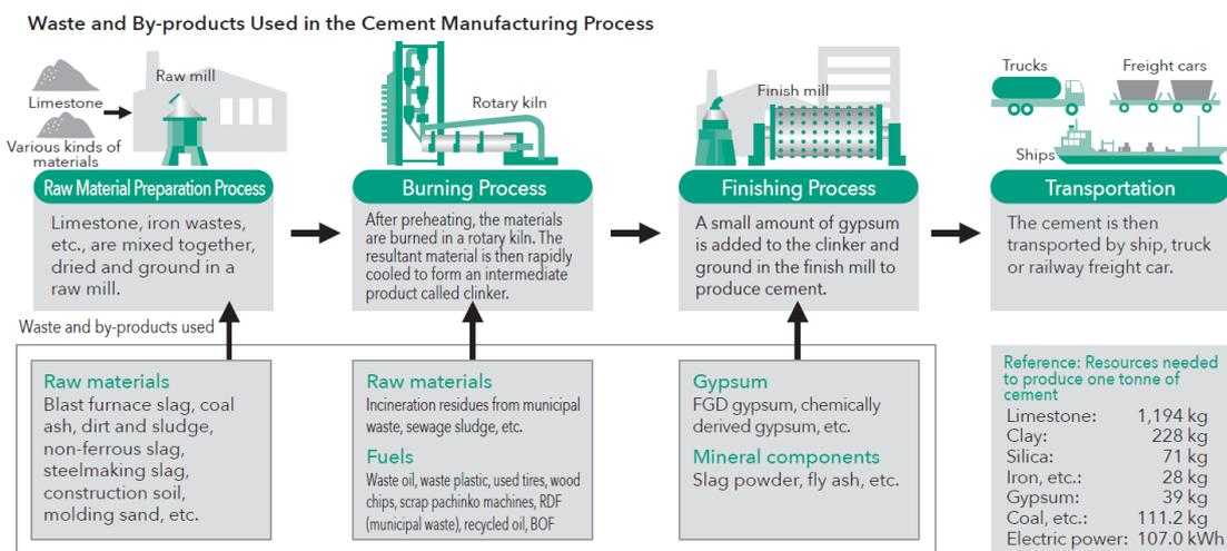
Fig. 1 Waste and by-products used in the cement manufacturing process
