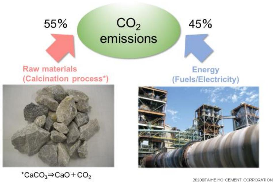
Fig. 2 CO<sub>2</sub> emissions from cement production
