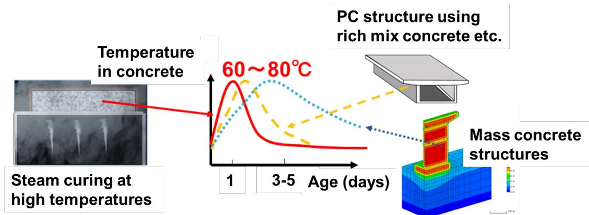
Figure-1 Types of concrete experiencing high temperatures
