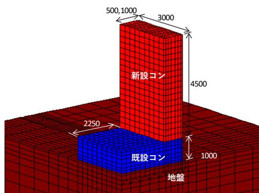
Figure-2 Mesh geometry of target structure
