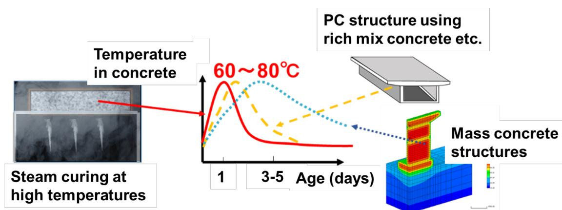
Figure-1 Types of concrete experiencing high temperatures
