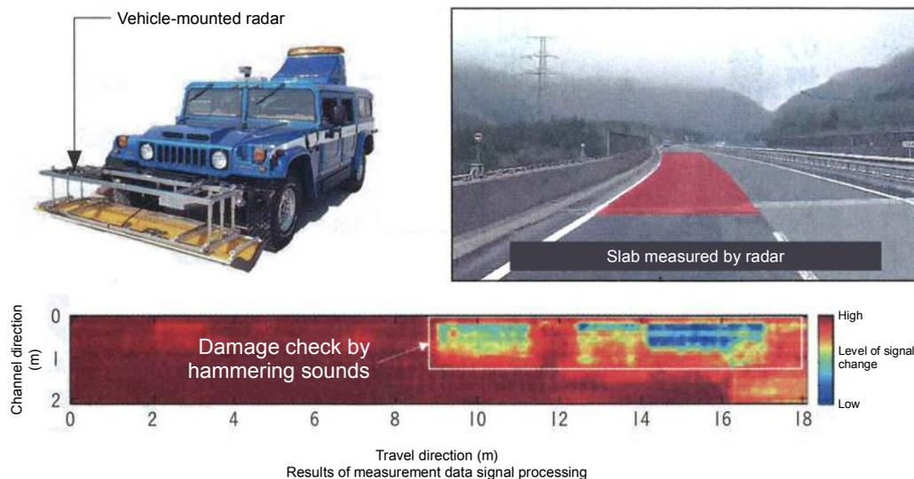
Fig. 1. Example of screening technology (3-D ground penetrating radar)
