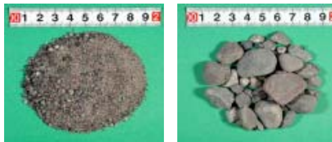
Figure 2. Recycled aggregates by heating and rubbing method
