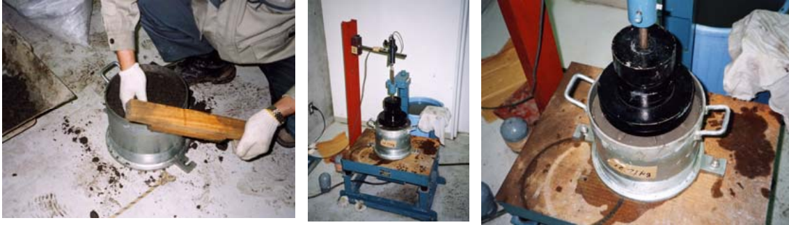
Photo 1 VC value testing machine
