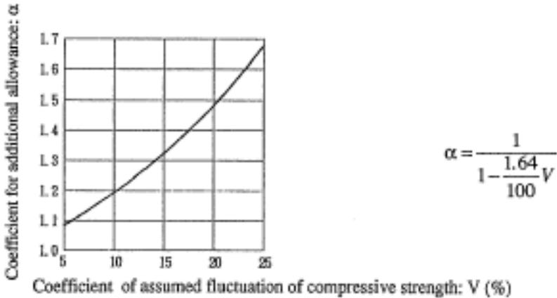
Fig. 4.3.1 Additional allowance & coefficient of antiwashout underwater concrete
