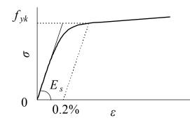
Figure C2.2.1 Definition of yield strength of stainless steel bars
