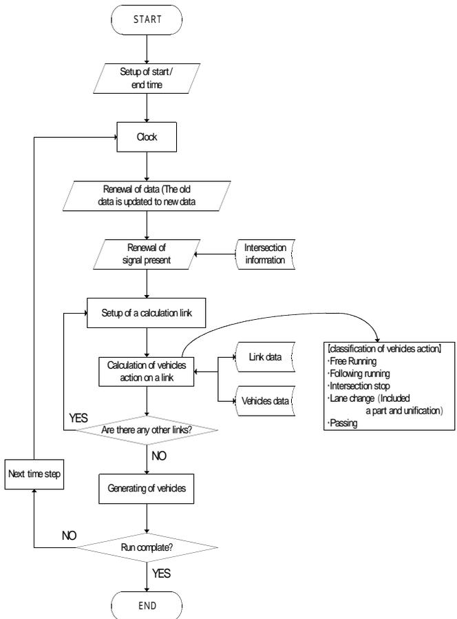
**Fig. 3** Simulation flow of Simr
