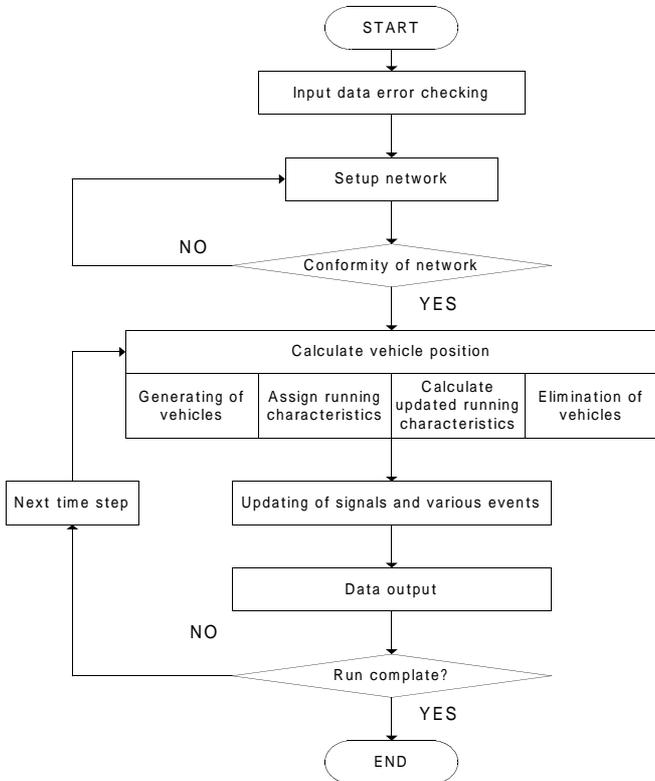
**Fig. 2** Simulation flow of NETSIM
